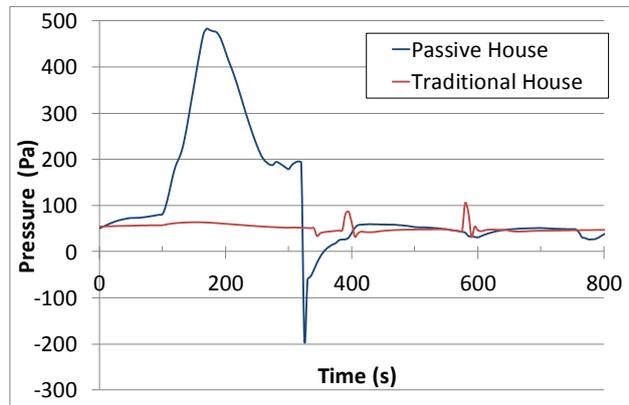
Figure 6: Fire-induced overpressure, (Brohez, 2012)
