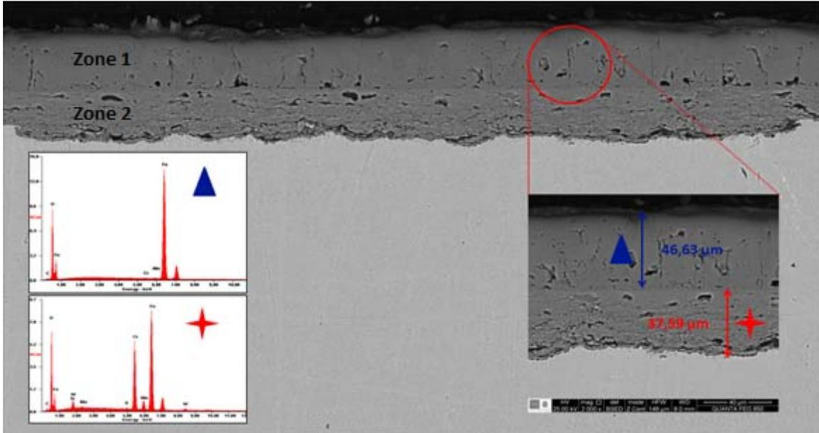
Figure 3: SEM-EDS from P92 sample after 360 h at 850 °C
