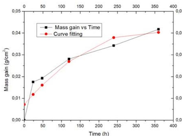
Figure 6: P92 mass gain against testing times
