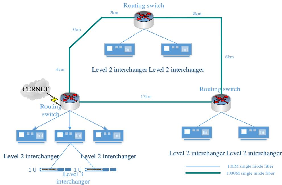
Figure 1: Chemical enterprise network backbone topology
