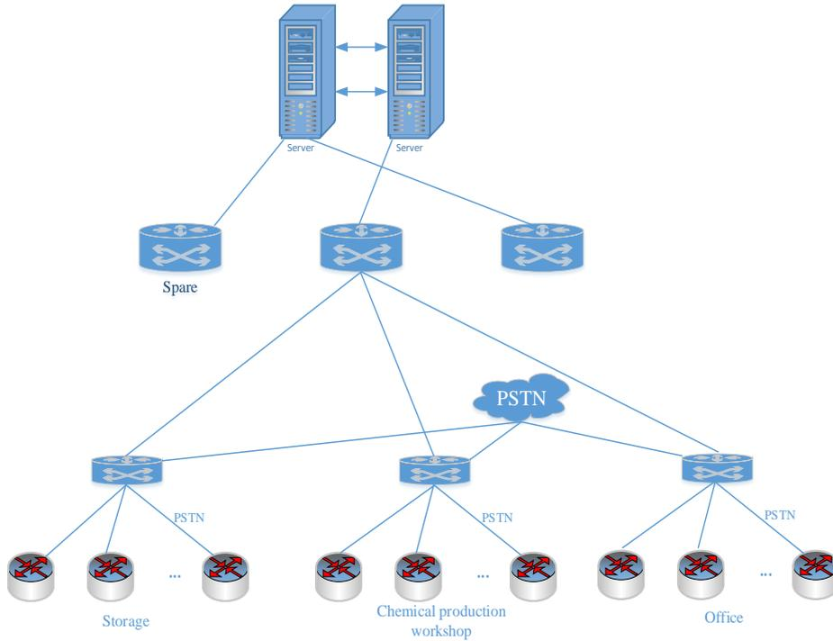
Figure 2: Hierarchical design network topology
