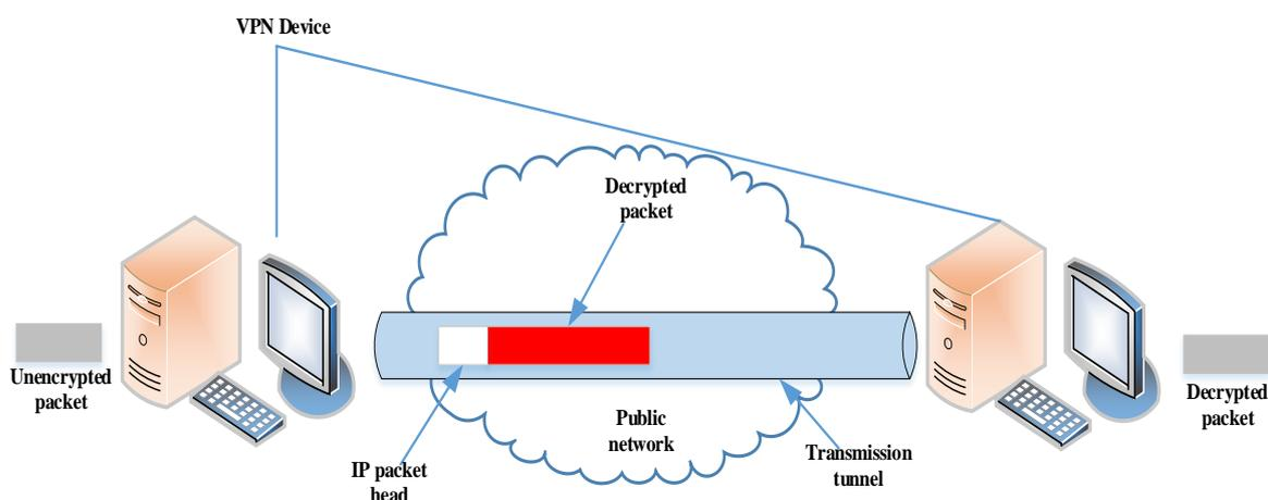
Figure 4: The VPN technology schematic
