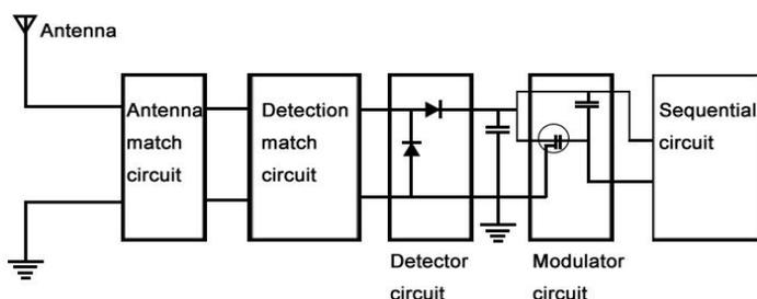
Figure 1: Working principle of electrical tags
