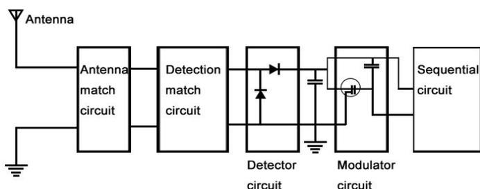
Figure 1: Working principle of electrical tags
