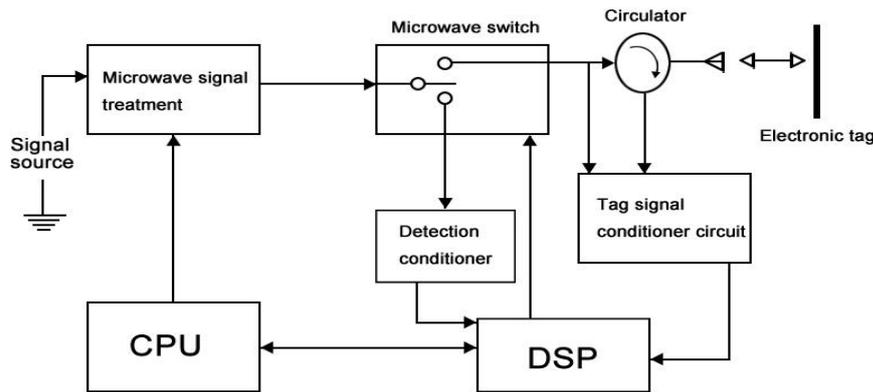
Figure 2: Working principle of reader-writer
