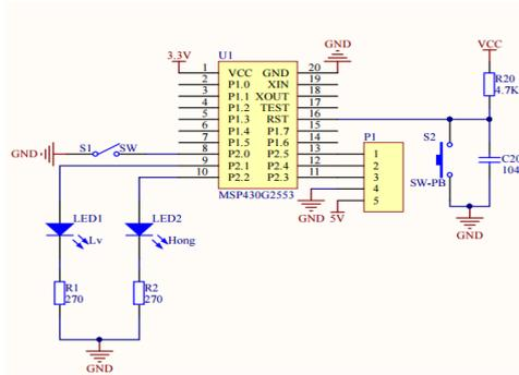
Figure 4: Schematic diagram of min system MSP430G2553
