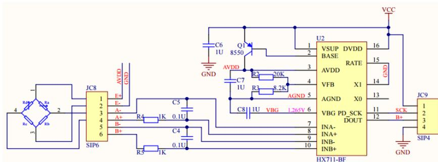
Figure 6: Working principle of sensor HX711 peripherals
