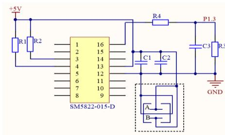
Figure 5: Schematic diagram of SM5822-015-D peripherals
