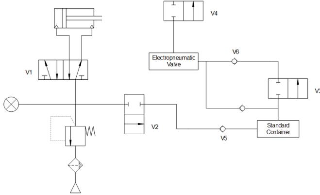
Figure 1: Schematic diagram of pneumatic circuit
