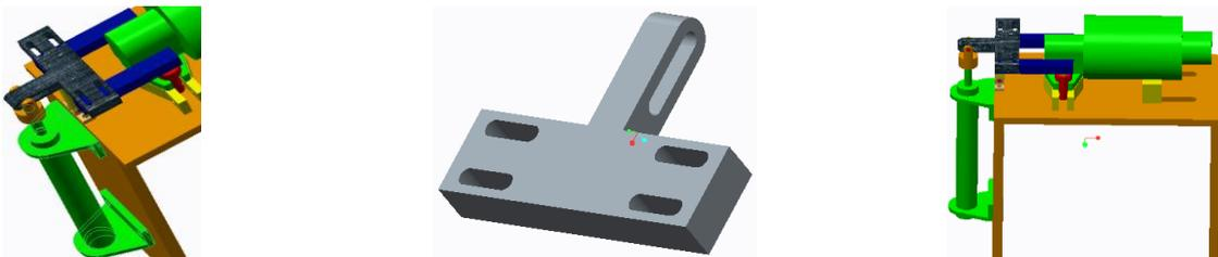
Figure 3: 3D map of electropneumatic valve clamps, (a) Clamp mechanism (b) Spacing adjustable beam (c) Fixture assembly
