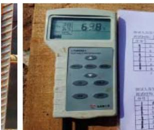
Figure 2: The temperature sensor and handheld temperature readout
