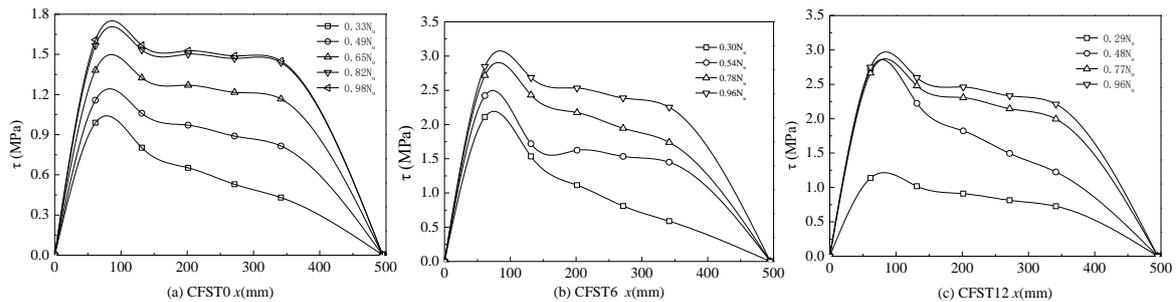
Figure 7: Curve of interfacial bond stress as a function of specimen height  $x$
