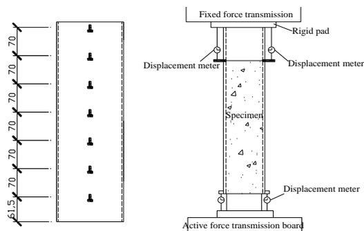
Figure 1: Layout of strain and displacement survey station
