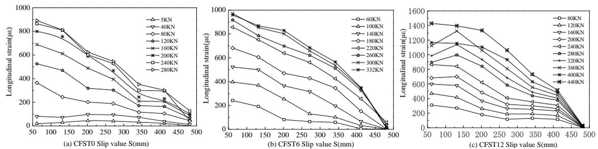
Figure 4: Longitudinal strain distribution on the surface of specimen
