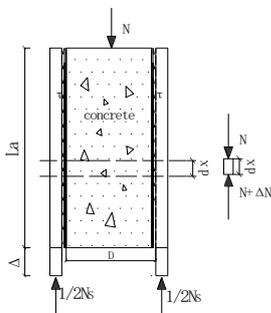
Figure 2: Test apparatus and mechanical model
