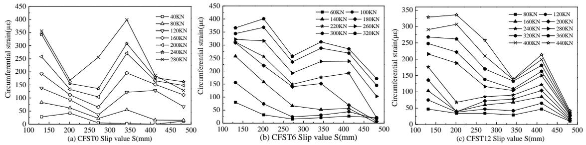
Figure 5: Circumferential strain distribution on the surface of specimen
