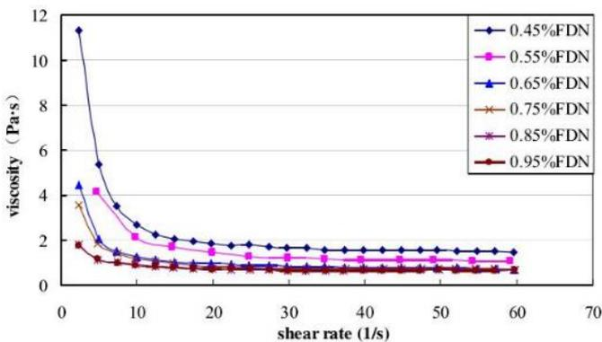
Figure 2: Shear rate - Plastic viscosity curve at 5 minutes with FDN cement paste
