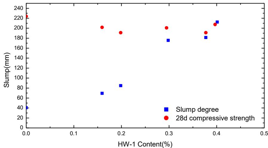
Figure 5: Slump and strength were correlated with the amount of HW-1
