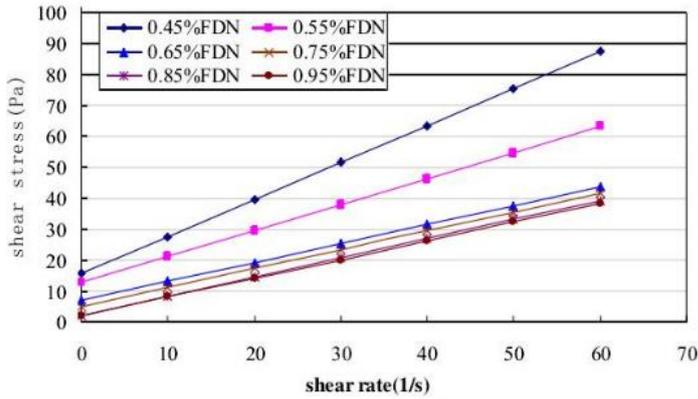
Figure 3: The Bingham curve of FDN cement paste at 5 minutes
