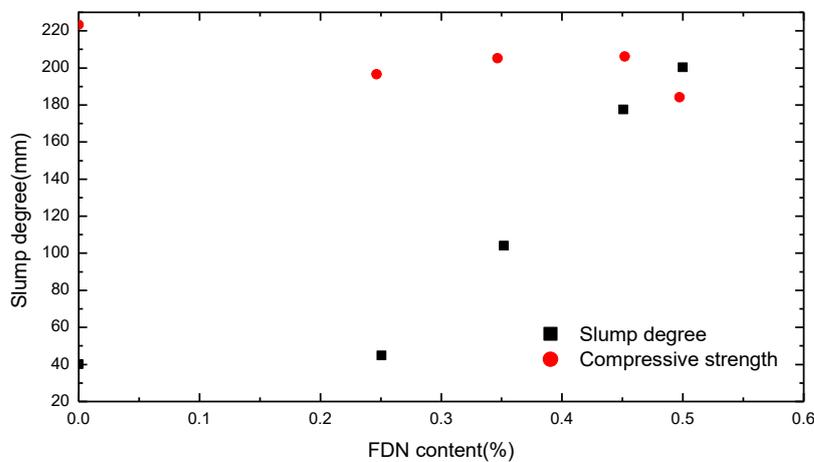
Figure 4: Slump and strength were correlated with FDN content
