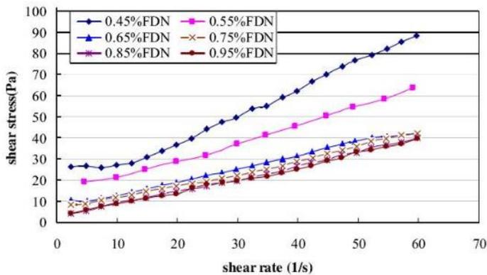
Figure 1: Shear Rate - Shear stress curve of FDN cement paste at 5 minutes
