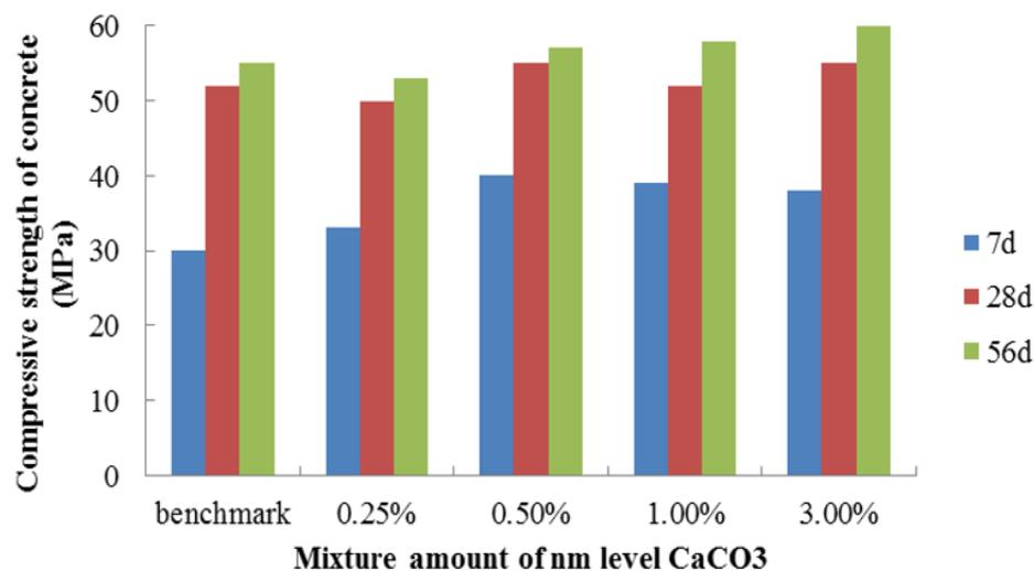
Figure 3: Compressive strength of concrete after NC and 2%SF incorporation
