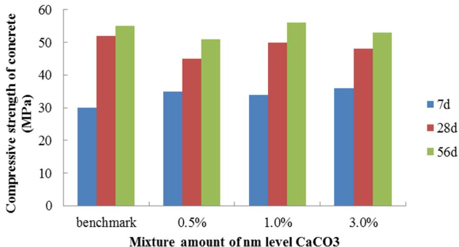
Figure 1: Compressive strength of concrete after NC incorporation
