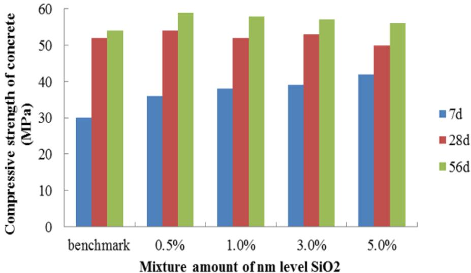
Figure 2: Compressive strength of concrete after NS incorporation
