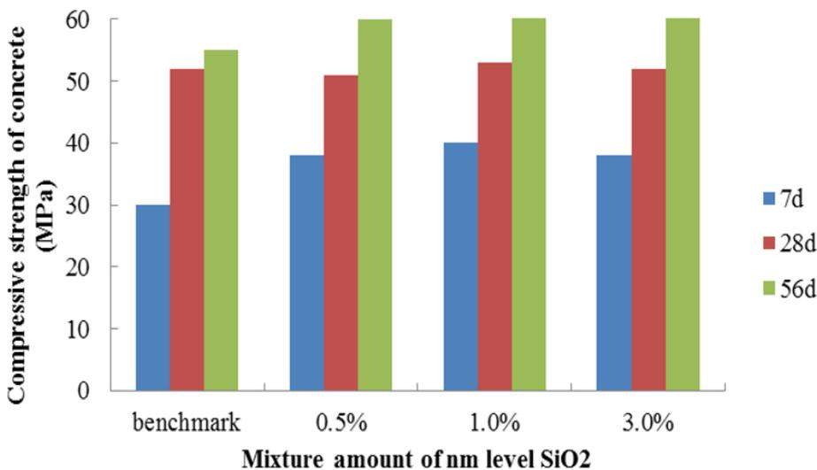
Figure 5: Compressive strength of concrete after NC and NS incorporation
