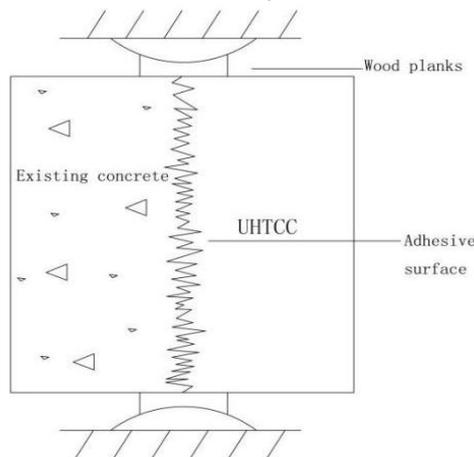
Figure 2: Tensile test device
