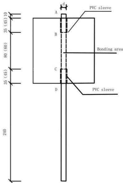
Figure 5: Details of the test
