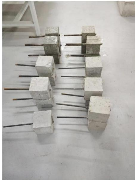
Figure 6: Pull-out test specimens
