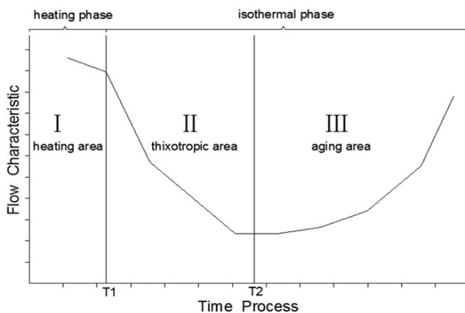
Figure 1: Flow Characteristics of Cast Asphalt Mixture with the Changing of Mixing Time
