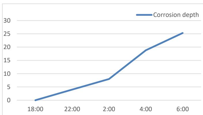
Figure 1: the trend curve of the inlet corrosion depth of the atmospheric tower top heat exchanger
