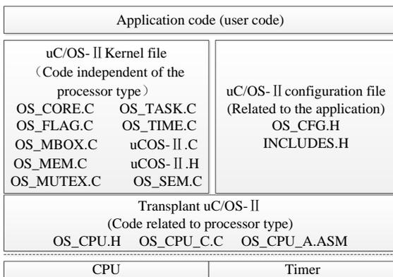
Figure 5: uC/OS-II file structure
