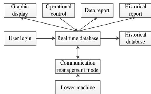
Figure 7: Real-time database transaction scheduling
