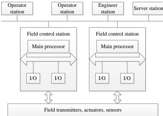
Figure 6: Typical distributed control system architecture
