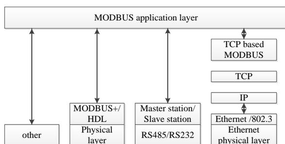
Figure 1: Modbus communication stack
