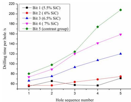
Figure 1: Drilling efficiency of bits
