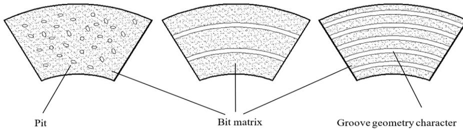
Figure 5: Sharpening effect of pits
