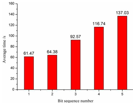
Figure 2: Average drilling time for single hole of every bit
