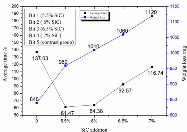
Figure 3: Average single-hole drilling time and wear weight loss
