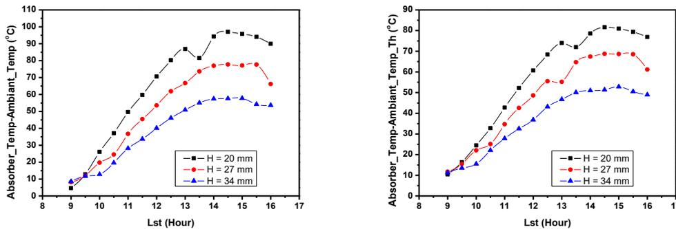
Figure 3: Evolution of the difference of theoretical and experimental temperature of the absorber as a function of time for different distances
