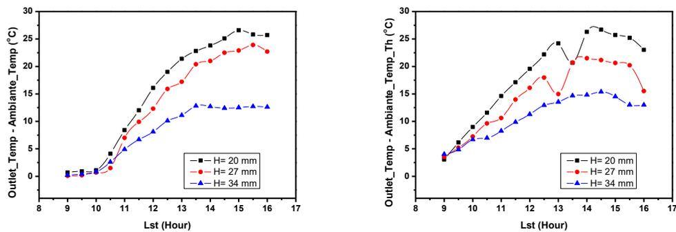
Figure 5: Evolution of the difference of theoretical and experimental outlet temperature as a function of time
