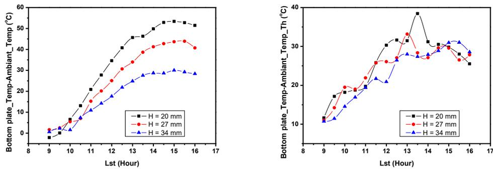
Figure 4: Evolution of the difference of theoretical and experimental temperature of the bottom plate as a function of time for different distances
