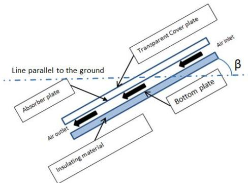
Figure 1: Cross-section of solar air collector with single pass of air
