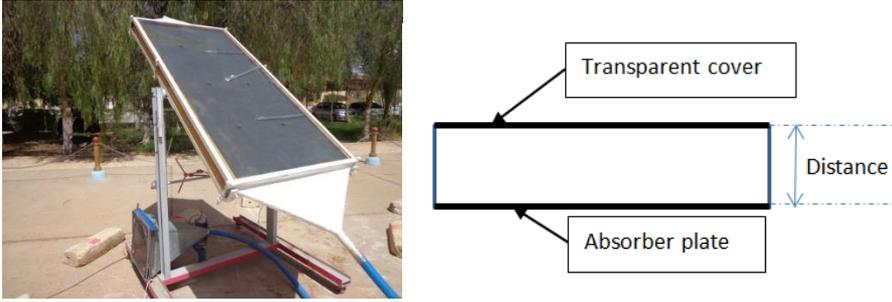
Figure 2: The photograph of experimental set-up and schematic description of the distance between the absorber and the transparent cover
