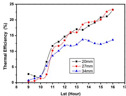
Figure 6: Evolution of thermal efficiency of the collector as a function of time for the three different distances
