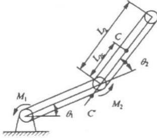
Figure 1: Schematic diagram of a horizontal 3R underactuated robot
