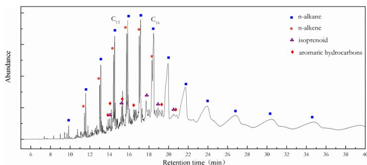
Figure 5: GC-MS spectrum of shale oil
