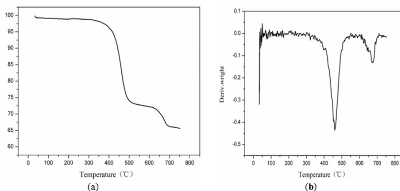
Figure 2: (a) Thermogravimetric (TG) curve of Huadian oil shale; (b) Derivative Thermogravimetric (DTG) curve of Huadian oil shale.
