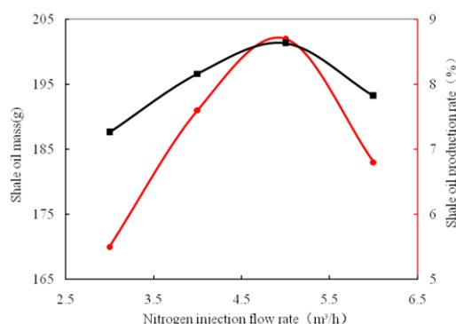
Figure 3: Shale oil mass and production rate along with nitrogen injection flow rate.
