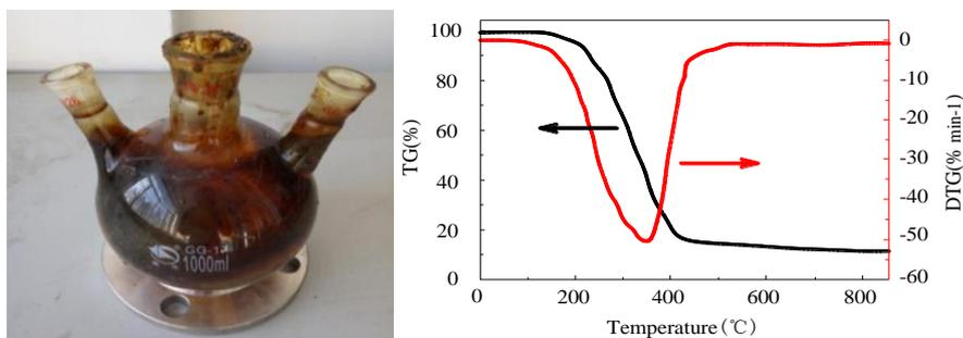
Figure 4: Shale oil and TG/DTG curves
