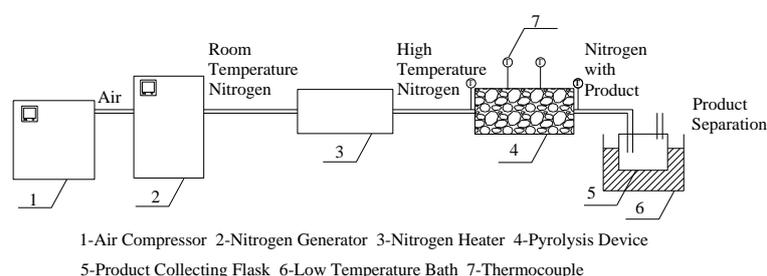
Figure 1: Principle of the pyrolysis experiment
