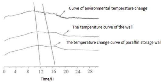
Figure 3: The response curve of temperature change of wall environment of phase-change energy storage building materials
