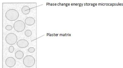
Figure 4: Profile of gypsum matrix phase-change energy storage material
