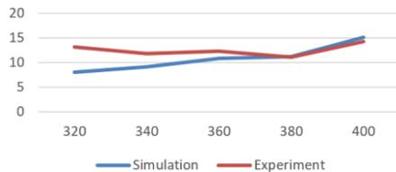
Figure 2: Comparison of grain size of AZ80 magnesium alloy at different extrusion temperatures
