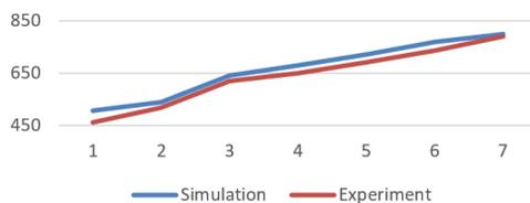
Figure 5: Extrusion force with different extrusion ratios
