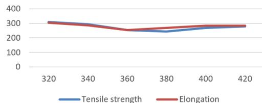
Figure 3: Mechanical properties of AZ80 alloy gland parts
