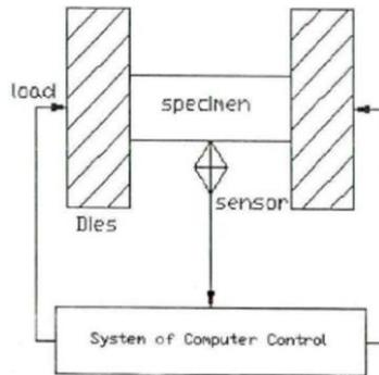
Figure 1: Experimental schematic
