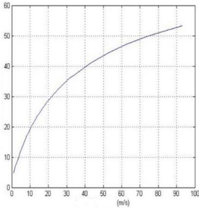
Figure3: Relationship between heat transfer coefficient (with plug-in) and air inlet wind speed
