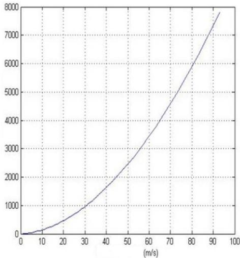
Figure 5: Relationship between air pressure drop (without plug-in tube) and inlet air speed
