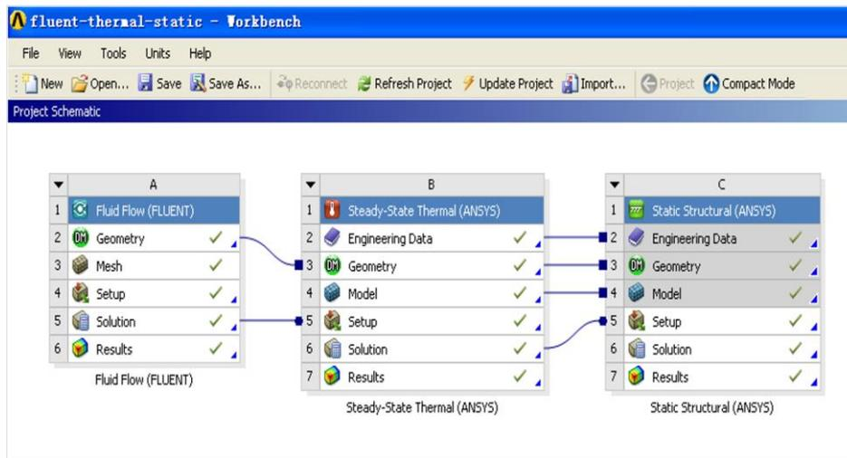
Figure 1: Co-simulation interface
