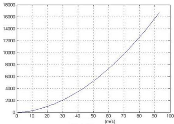
Figure 6: Relationship between air pressure drop (with plug-in tube) and inlet air speed
