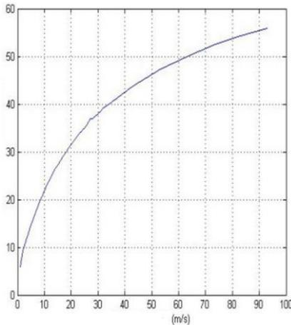
Figure 4: Relationship between heat transfer coefficient (without plug-in) and air inlet wind speed
