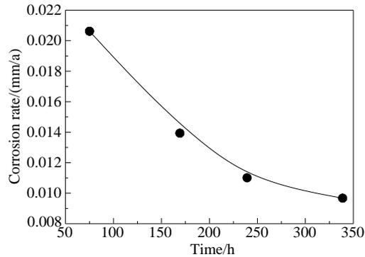
Figure 2: Average corrosion rate of multi-element copper alloys at different etching duration
