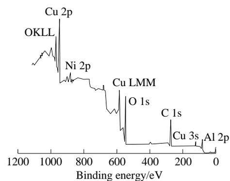
Figure 7: XPS spectra of corrosion products of multi-element copper alloys at pH=12
