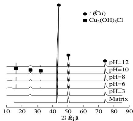
Figure 6: XRD spectra of corrosion products of multi-element copper alloy at different pH values
