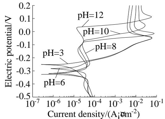
Figure 5: Polarization curves of multi-element copper alloys at different pH values
