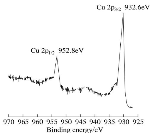
Figure 8: Cu2p narrow-spectrum analysis results of the multi-element copper alloy at pH=12
