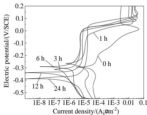
Figure 3: Polarization curves of multi-element copper alloys at different etching duration
