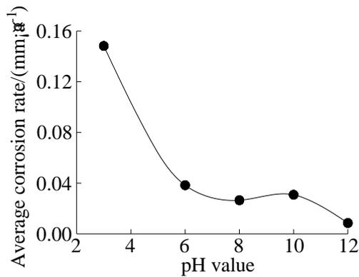
Figure 4: Average corrosion rate of multi-element copper alloys at different pH values
