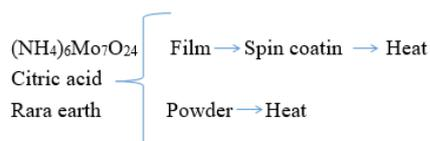
Figure 1: film and powder sample process
