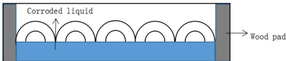
Figure 2: Schematic diagram of corrosion device
