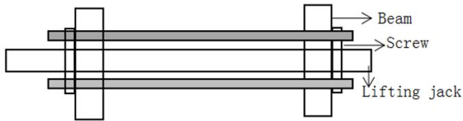
Figure 3: Test loading device
