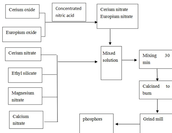
Figure 1: Preparation of a single matrix white led with fluorescent powder
