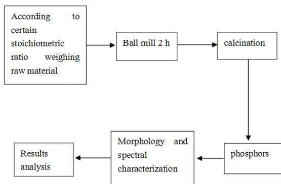
Figure 2: Preparation of a single matrix white LED with fluorescent powder
