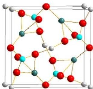
Figure 3: Schematic diagram of crystal structure of  $\text{Ca}_2\text{MgSi}_2\text{O}_7$
