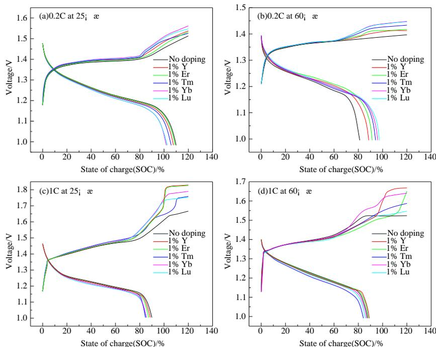
Figure 1: Charge-discharge curve of Ni-MH Batterie with REOs
