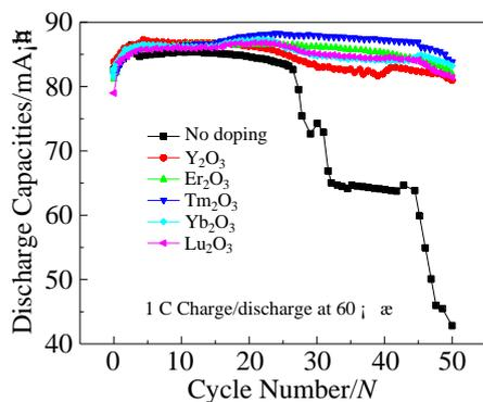
Figure 6: Service life of different types of Ni-MH Batteries at high temp
