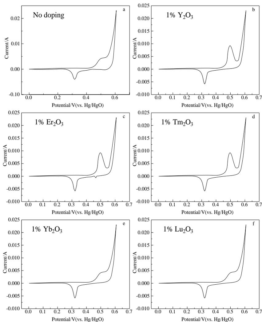
Figure 5: Curve of volt-ampere characteristics of different types of Ni-MH batteries at high temp
