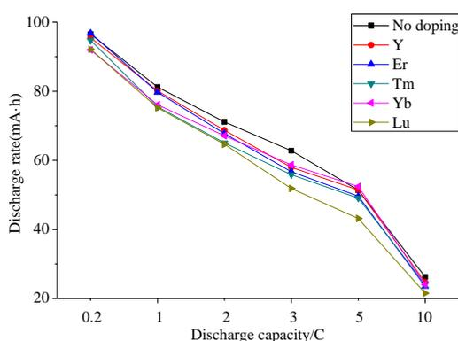
Figure 2: Discharge capacity of different types of Ni-MH Batteries at 0.2~10C at room temp
