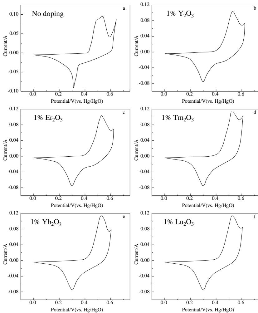
Figure 4: Curve of volt-ampere characteristics of different types of Ni-MH Batteries at room temp.
