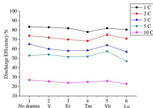
Figure 3: Discharge efficiency of different types of Ni-MH Batteries at 0.2~10C at room temp
