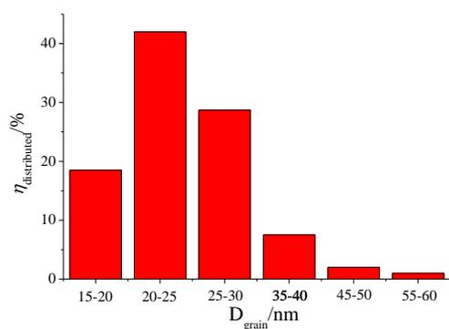
Figure 4: Statistics of nano copper particle size distribution
