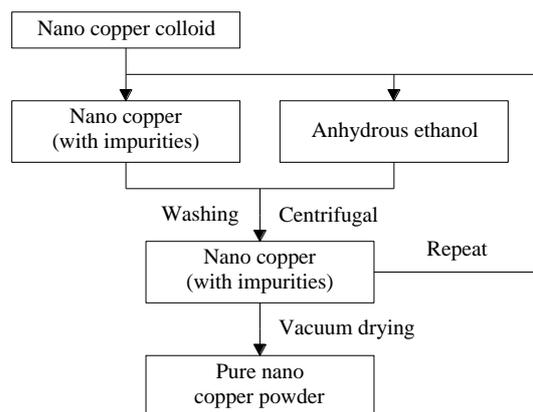
Figure 2: Preparation process of nano-copper powder
