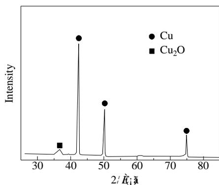
Figure 3: X-ray diffraction pattern of nano copper powder
