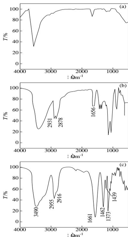
Figure 5: Infrared spectrum analysis of nano copper powder and PVP
