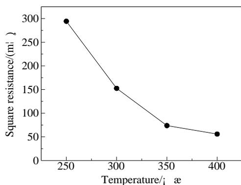
Figure 7: Curve of sheet resistance of nano-copper conductive ink as a function of sintering temperatures (sintered for 15 min)
