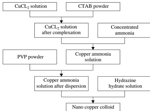
Figure 1: Preparation process of nano-copper colloids
