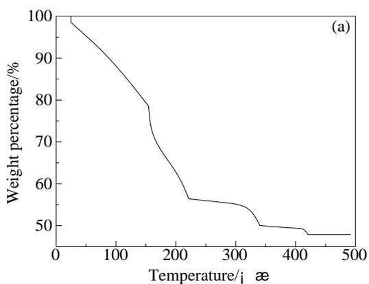
Figure 6: Thermogravimetric curve of nano copper conductive ink
