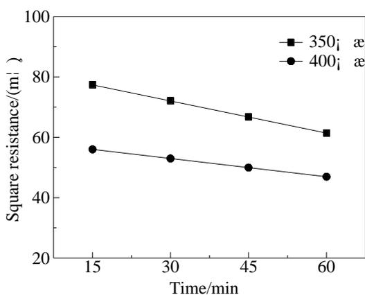
Figure 8: Curve of sheet resistance of nano copper conductive ink as a function of sintering time
