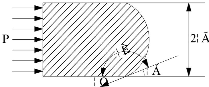
Figure 1: Force on mercury inside the pores
