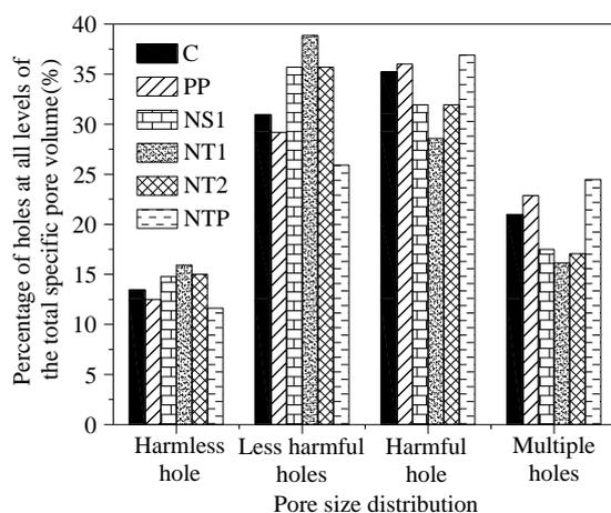
Figure 3: Distribution of internal pore with different diameters of different types of concrete
