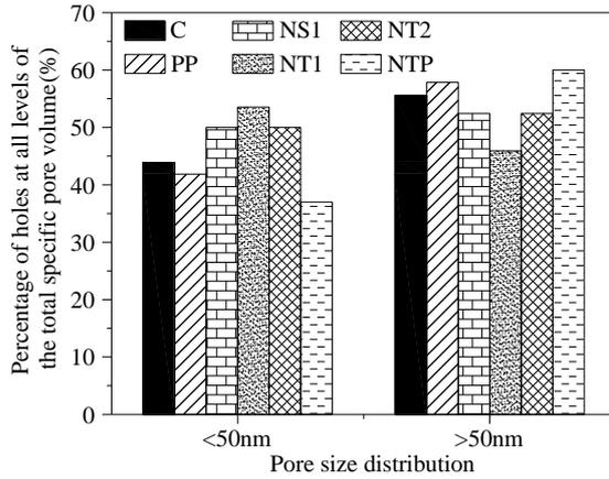
Figure 4: Distribution of internal pores with diameters less than 50 nm and that greater than 50 nm of different types of concrete
