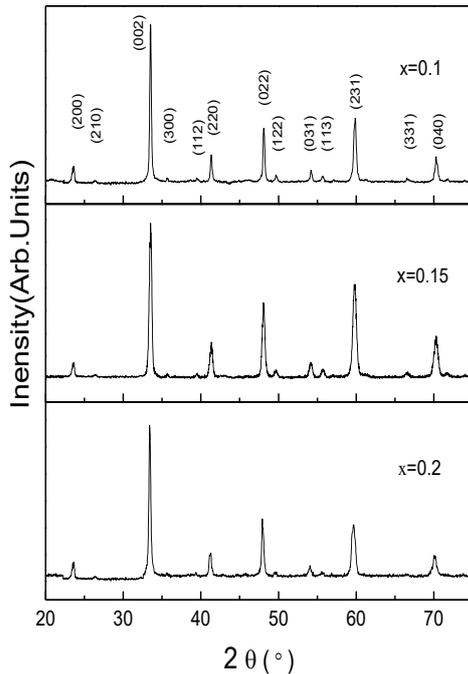
Figure 1: The room temperature X-ray diffraction pattern of  $\text{Nd}_{1-x}\text{Sr}_x\text{CoO}_3$  ( $x=0.10, 0.15, 0.20$ )
