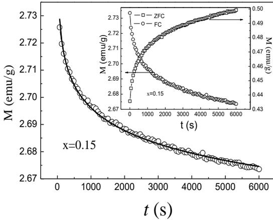
Figure 3: The remanent magnetization of  $Nd_{1-x}Sr_xCoO_3$  ( $x=0.15$ ). The solid line is the best fits Eq. 1
