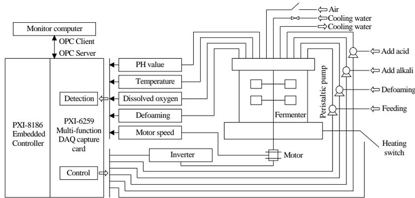
Figure 2: Hardware design framework of bio-fermentation intelligent monitoring system
