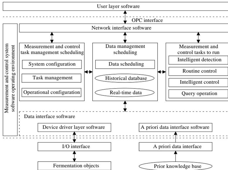
Figure 3: Software design framework of bio-fermentation intelligent monitoring system
