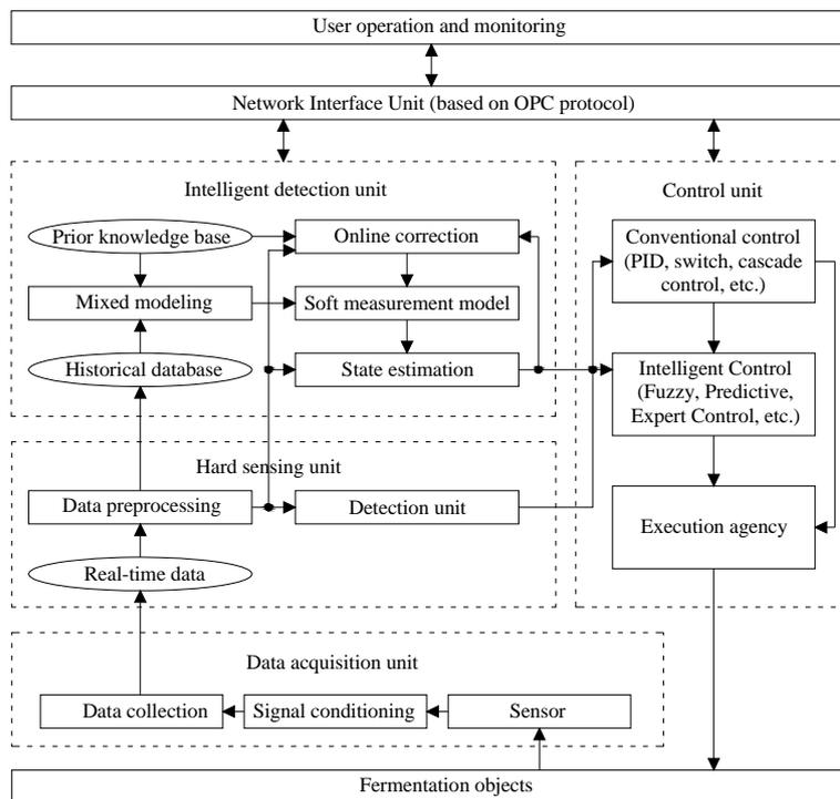
Figure 1: Overall architecture of bio-fermentation intelligent monitoring system
