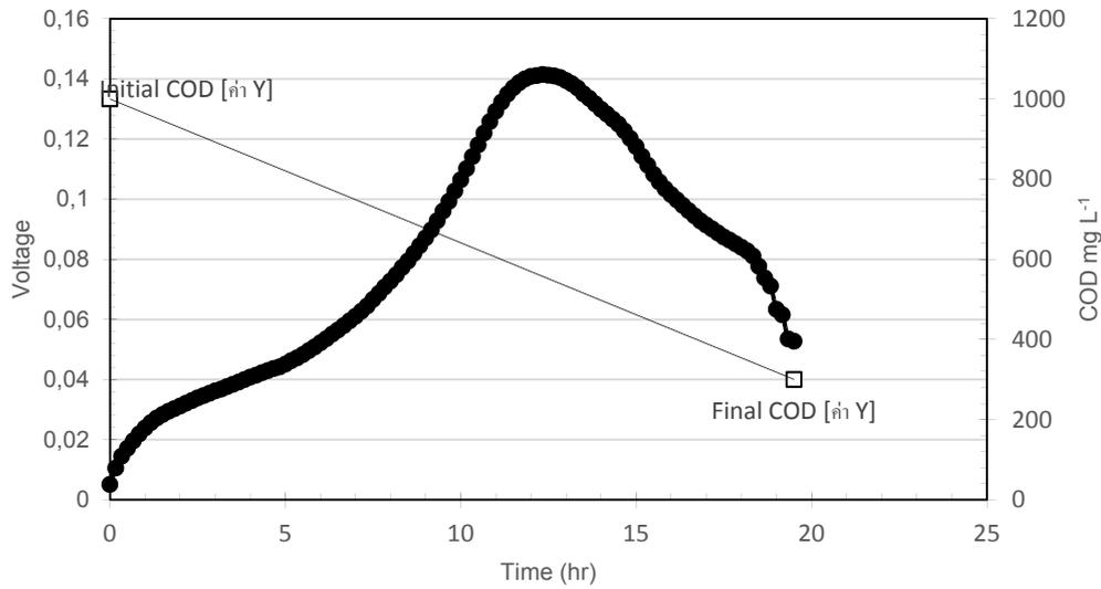
Figure 3: The relationship between voltage and COD removal from tannery wastewater in MFC.
