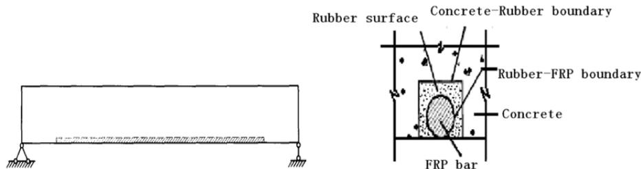
Figure 2: Plan for embedded FRP reinforcement
