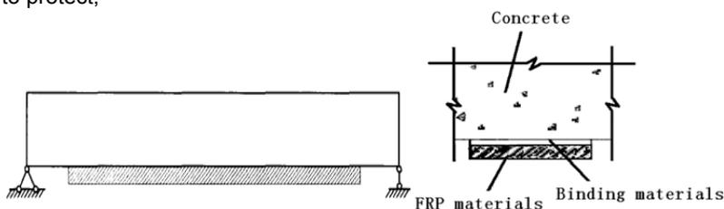
Figure 3: Plan for external bonding
