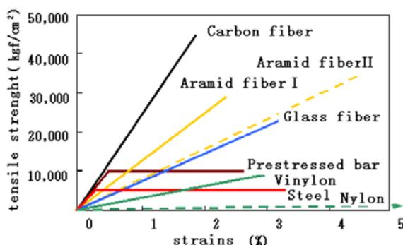
Figure 1: Mechanical performance comparison of FRP with other fibre materials
