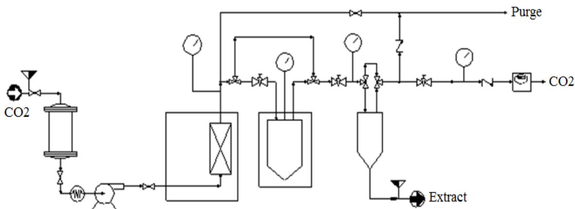
Figure 2: Example of a SC- $\text{CO}_2$  extraction plant layout.
