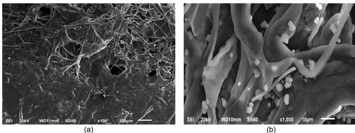
Figure 2: SEM of collagen from “Kacang” goat skin (a) scale bar 100  $\mu\text{m}$ , (b) scale bar 10  $\mu\text{m}$
