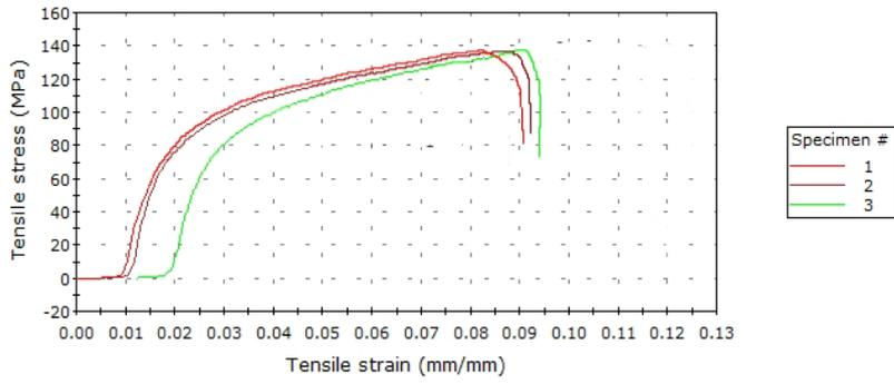
Figure 3: Tensile stress-strain plots for the composite samples with 0 wt% of SiCp loading
