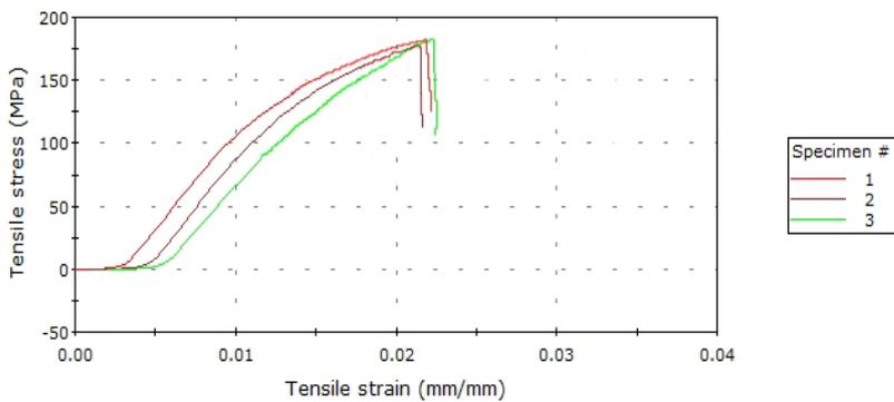
Figure 6: Tensile stress-strain plots for the composite samples with 30 wt% of SiCp loading
