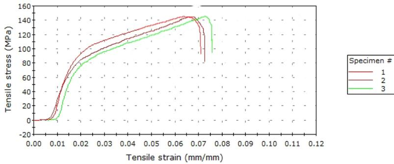
Figure 4: Tensile stress-strain plots for the composite samples with 10 wt% of SiCp loading
