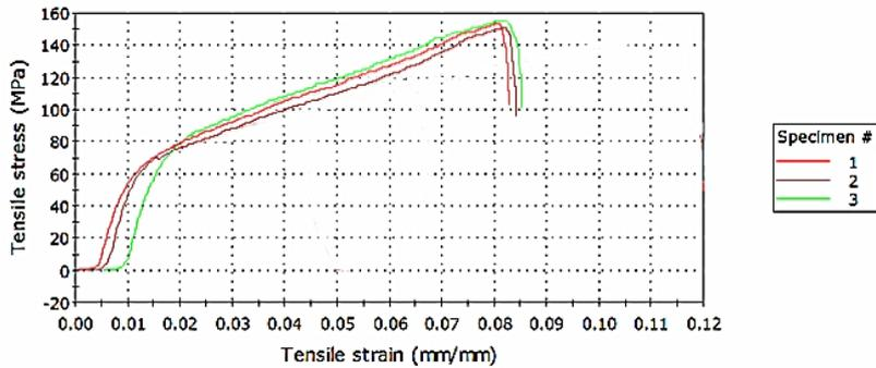
Figure 5: Tensile stress-strain plots for the composite samples with 20 wt% of SiCp loading
