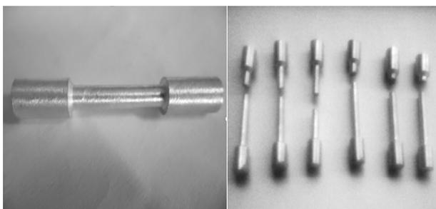
Figure 1: Tensile Strength Sample before and after test
