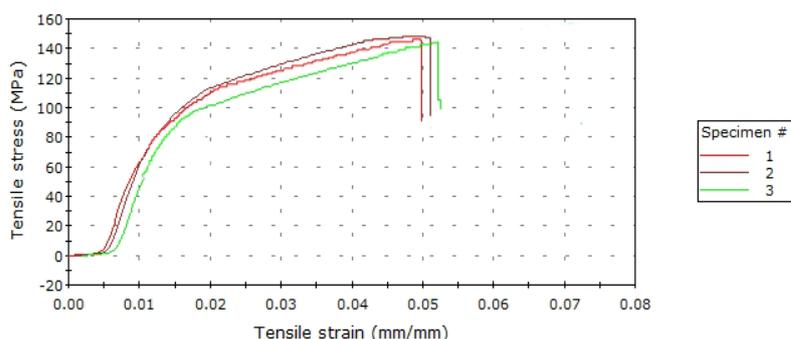
Figure 7: Tensile stress-strain plots for the composite samples with 50 wt% of SiCp loading
