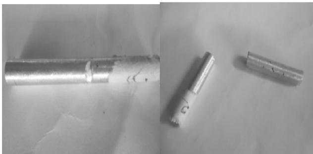
Figure 2: Notched specimen just before and after the impact (Izod) test
