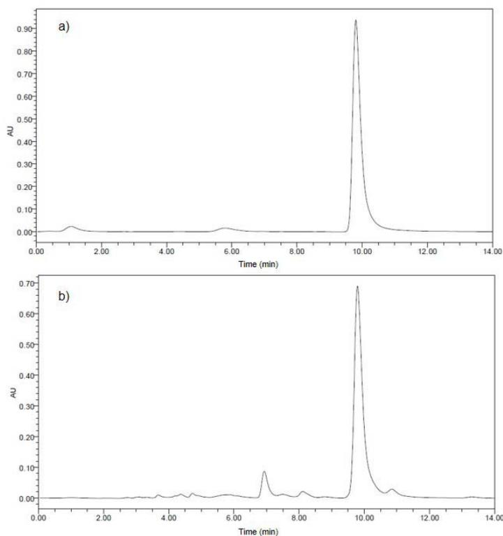
Figure 3: HPLC chromatogram profile for (a) standard of  $\alpha$  mangostin (b) one extract of  $scCO_2$
