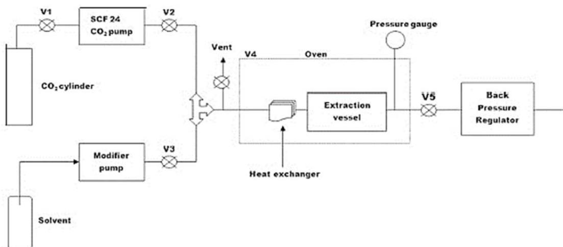
Figure 2: Schematic diagram of the SC-CO<sub>2</sub> extractor (Courtesy of CLEAR UTM Skudai)
