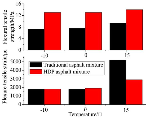
Figure 4: The bending-resistance strength and strain of traditional pitch and HDP mixed pitch
