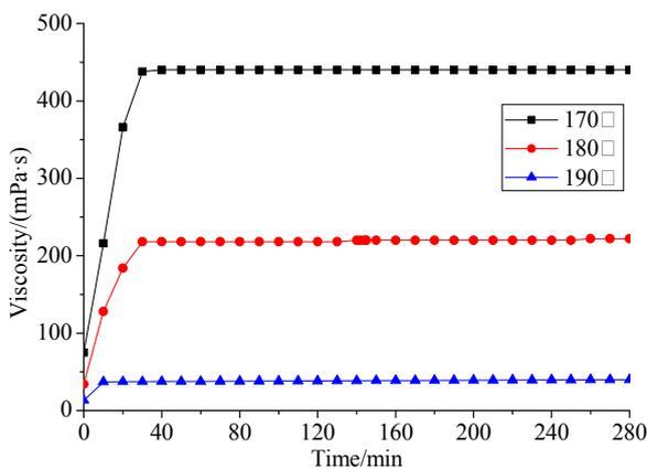
Figure 1: Viscosity curve between HDP and traditional pitch in different temperature
