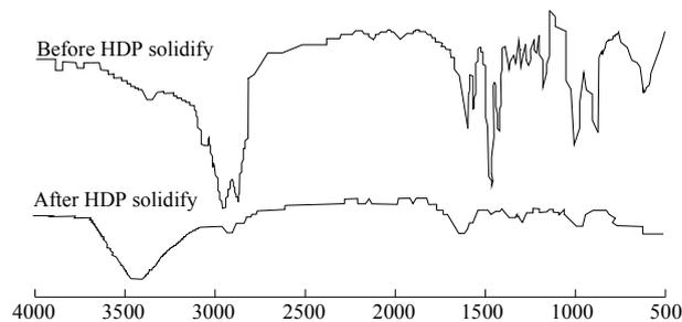
Figure 2: Infrared spectrum before and after HDP solidification
