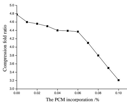
Figure 5: The FSPCM content for the effect of compression flexure ratio
