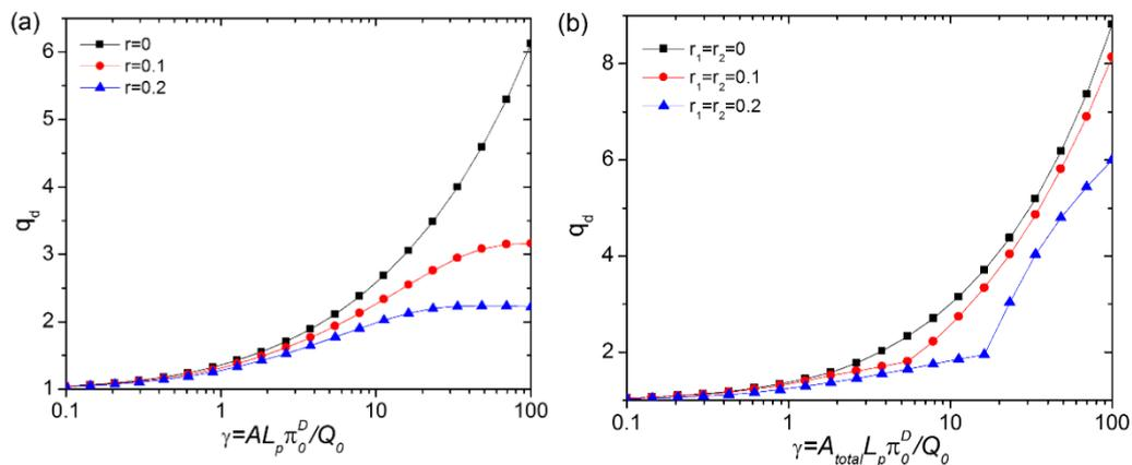
Figure 4: Optimal  $q_d$  in (a) a single-stage PRO and (b) a dual-stage PRO. The log scale is used in x-axis in the plots
