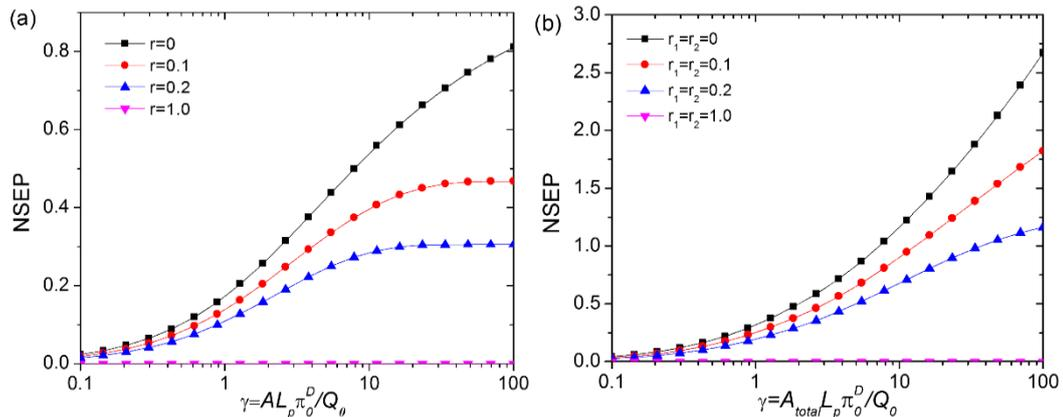
Figure 3: Optimal NSEPs in (a) a single-stage PRO and (b) a multi-stage PRO as a function of  $\gamma$  and  $r$ . The log scale is used in x-axis in the plots
