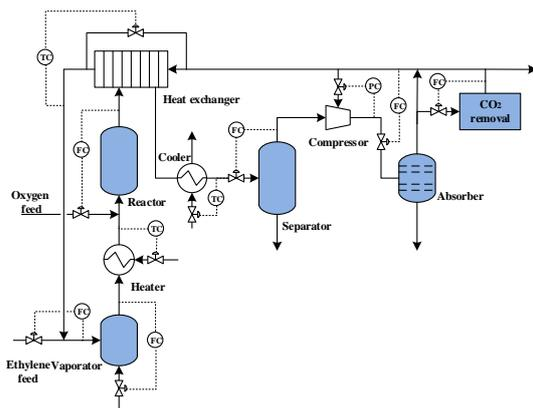
Figure 3: The control structure of part of process networks evolved in the fast time scale
