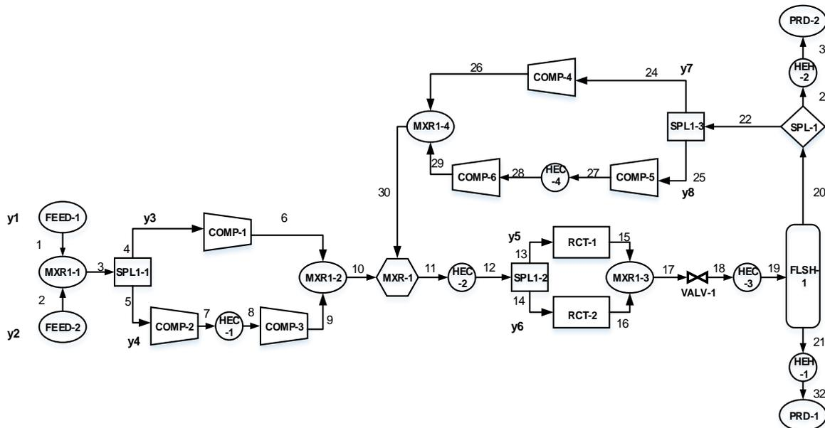
Figure 1: Superstructure for methanol process synthesis (modified from Kasaš et al, 2012)
