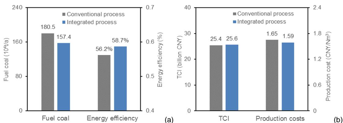
Figure 5: (a) Fuel coal consumption and energy efficiency; (b) Total cost investment and production costs
