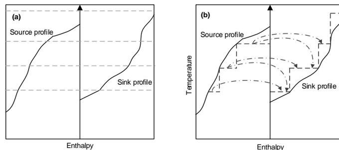
Figure 2: (a) Total Site Profiles with steam levels. (b) Total Site Profiles with potential steam heat recovery.
