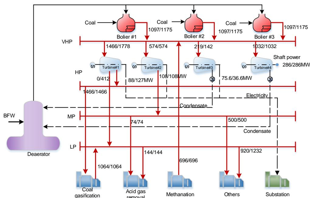
Figure 4: The utility system of the integrated process
