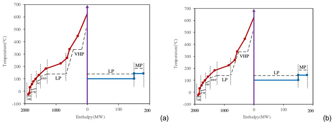
Figure 3: (a) The Total Site Profiles of conventional process; (b) The Total Site Profiles of integrated process
