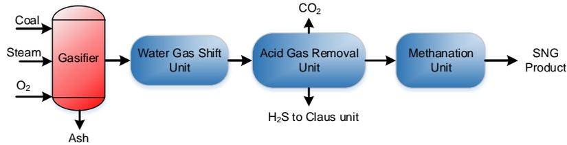
Figure 1: The general scheme of coal-based SNG process
