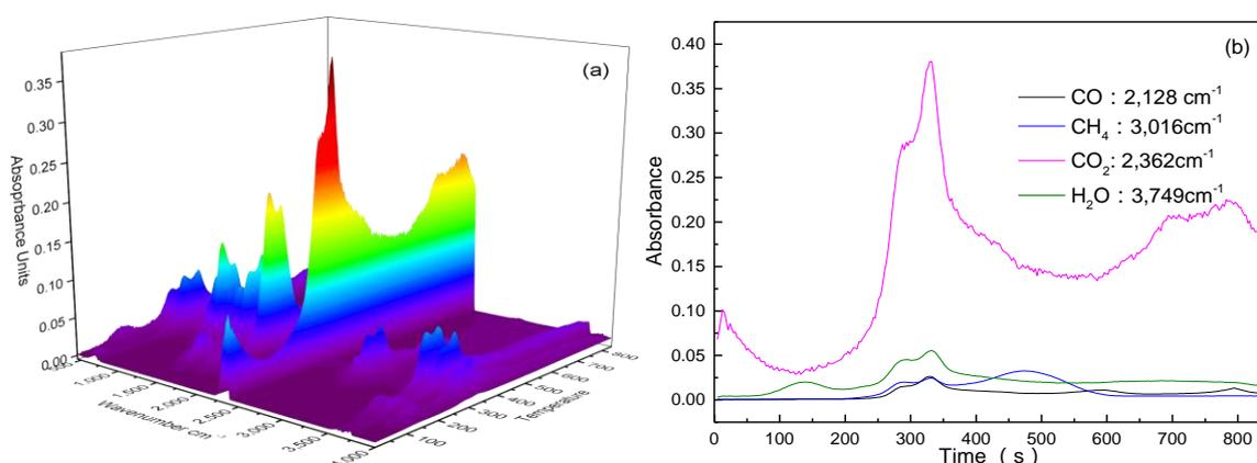
Figure 3: TG-FTIR analysis of evolved gases from the pyrolysis of straw at 70 °C/min (a) FTIR analysis of evolved gases (b) The evolved gases
