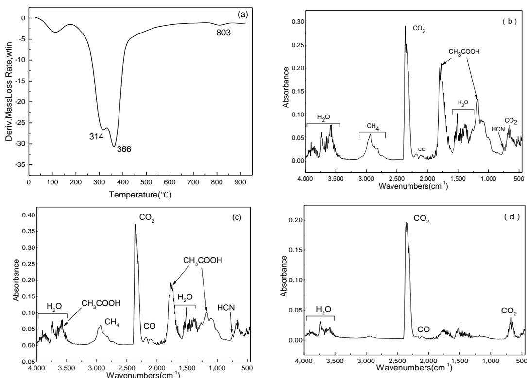
Figure 4: The FTIR spectra of straw pyrolysis: (a) DTG curve of straw at  $70^\circ\text{C}/\text{min}$ , (b) IR spectra at  $314^\circ\text{C}$ , (c) IR spectra at  $366^\circ\text{C}$ , and (d) IR spectra at  $803^\circ\text{C}$
