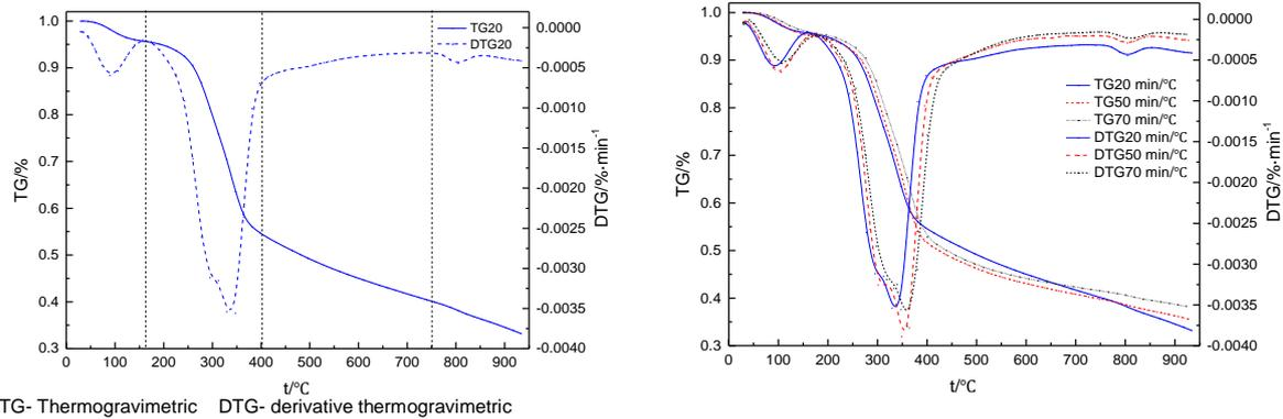
Figure 1: TG/DTG curves of straw: (a) Curves of Gasification Pyrolysis in 20 °C/min, (b) Weight loss Curves of Gasification Pyrolysis under Different Heating Rate
