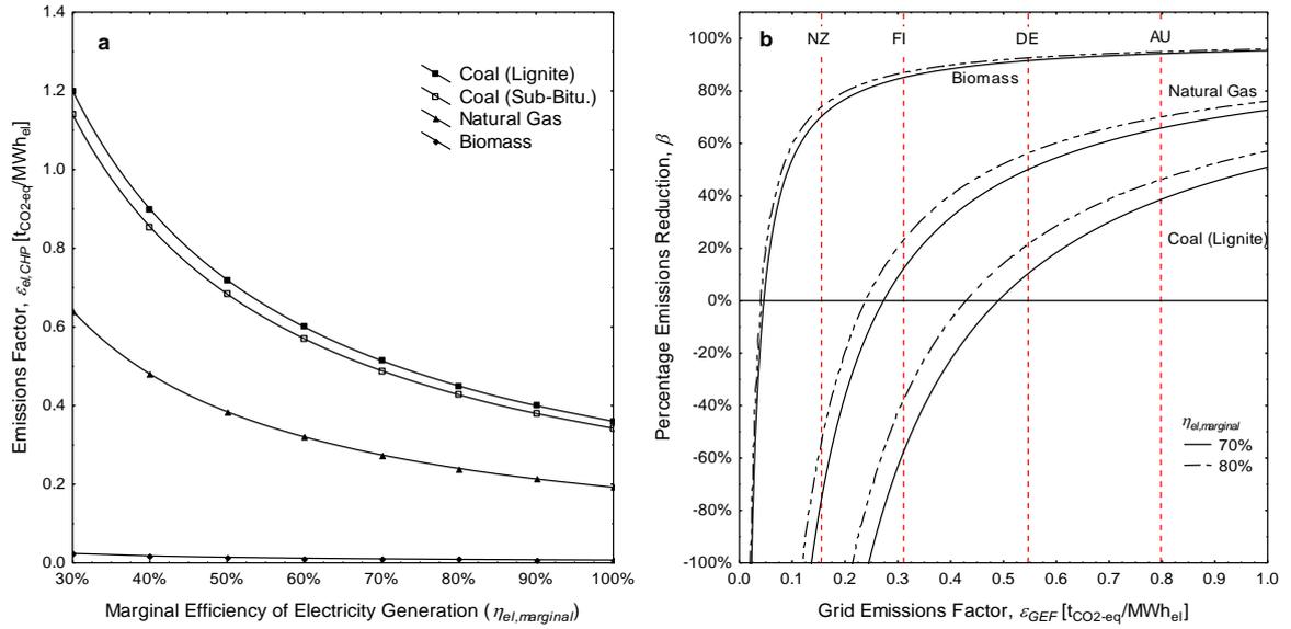
Figure 1: Emissions factor for CHP power generation (a) and percentage emissions reduction per unit of power generated using CHP (b).
