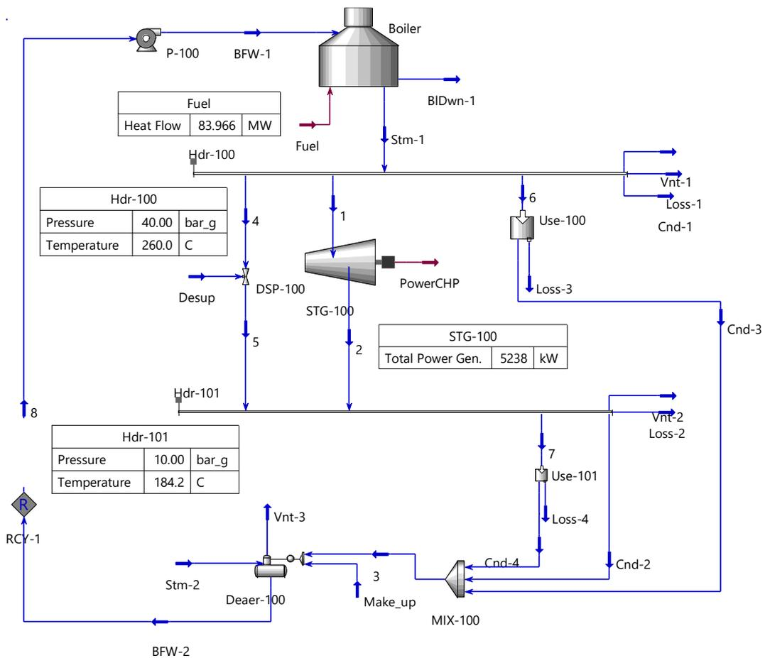
Figure 3: A typical example of a multi stage back pressure steam in use for CHP.
