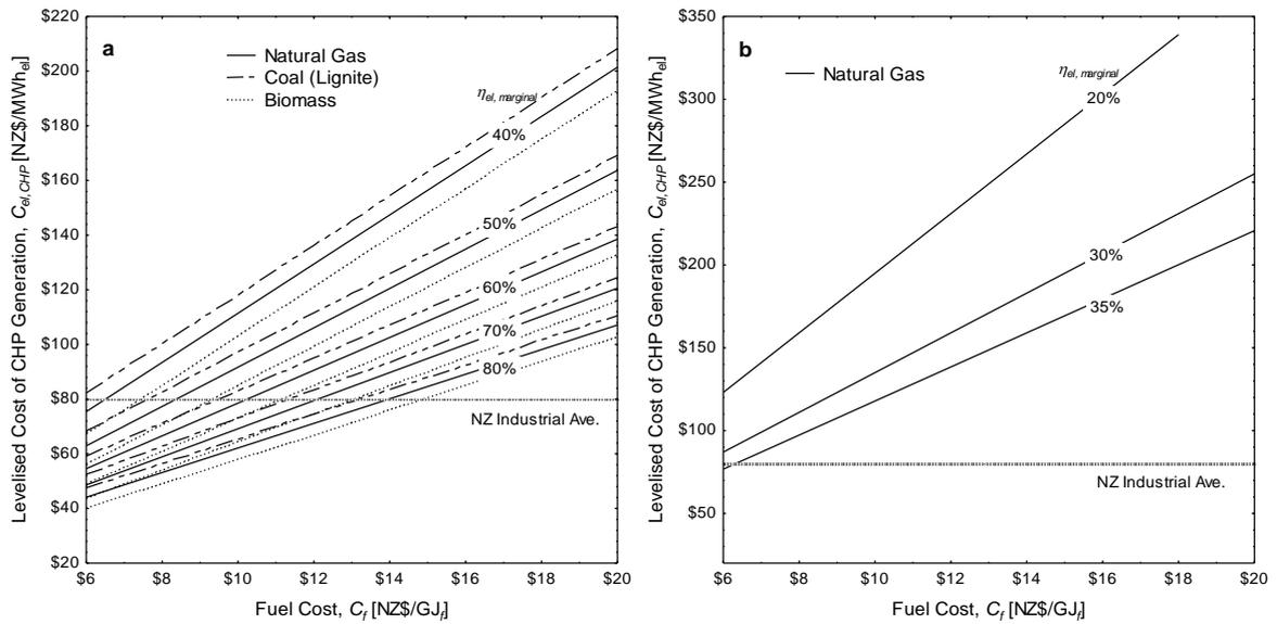
Figure 2: Levelised cost of power generation using back pressure steam turbines (a) and gas turbine (b) at different efficiency of electricity generation. A carbon price of NZ\$18/tCO<sub>2</sub>-eq is included.
