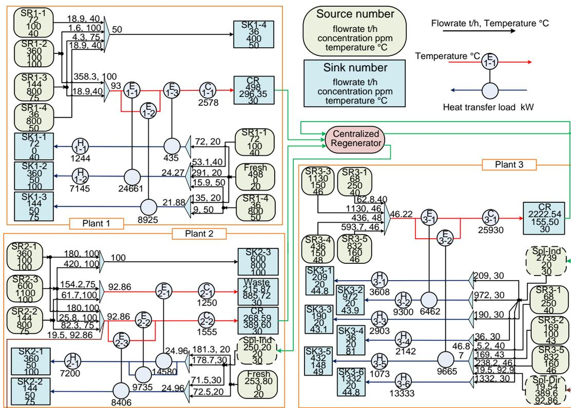
Figure 2: Optimal IHIWAN design of industrial park for case study
