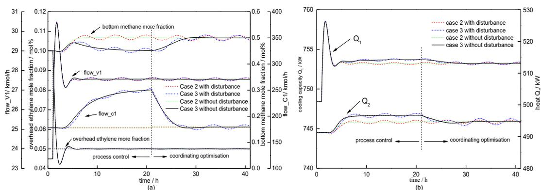
Figure 5: Changes of the demethaniser with and without disturbance; a) key mole fractions and flow rates at overhead and bottom; b) cooling capacity  $Q_1$  and heat  $Q_2$
