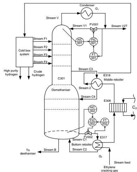
Figure 3: Flow sheet of the multi-feed demethaniser system
