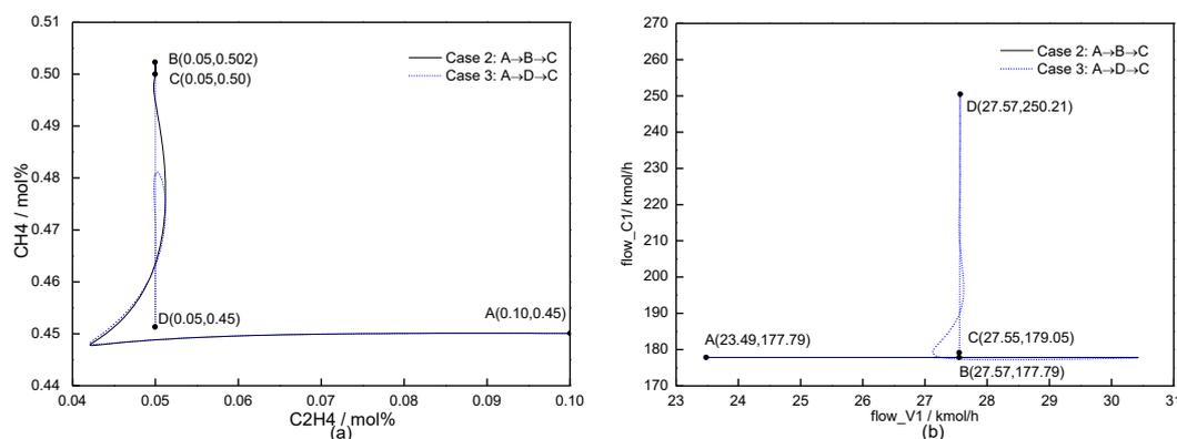
Figure 4: Dynamic relationships of the overhead and bottom key components and flow rates; a) overhead and bottom components of methane and ethylene; b) flow rates of Streams V1 and C1
