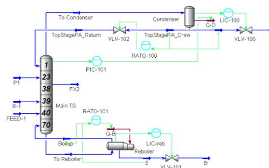
Figure 4: Sub-process configuration of ratio control (S3)
