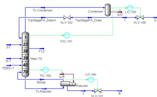
Figure 3: Sub-process configuration of pressure and temperature control (S2)
