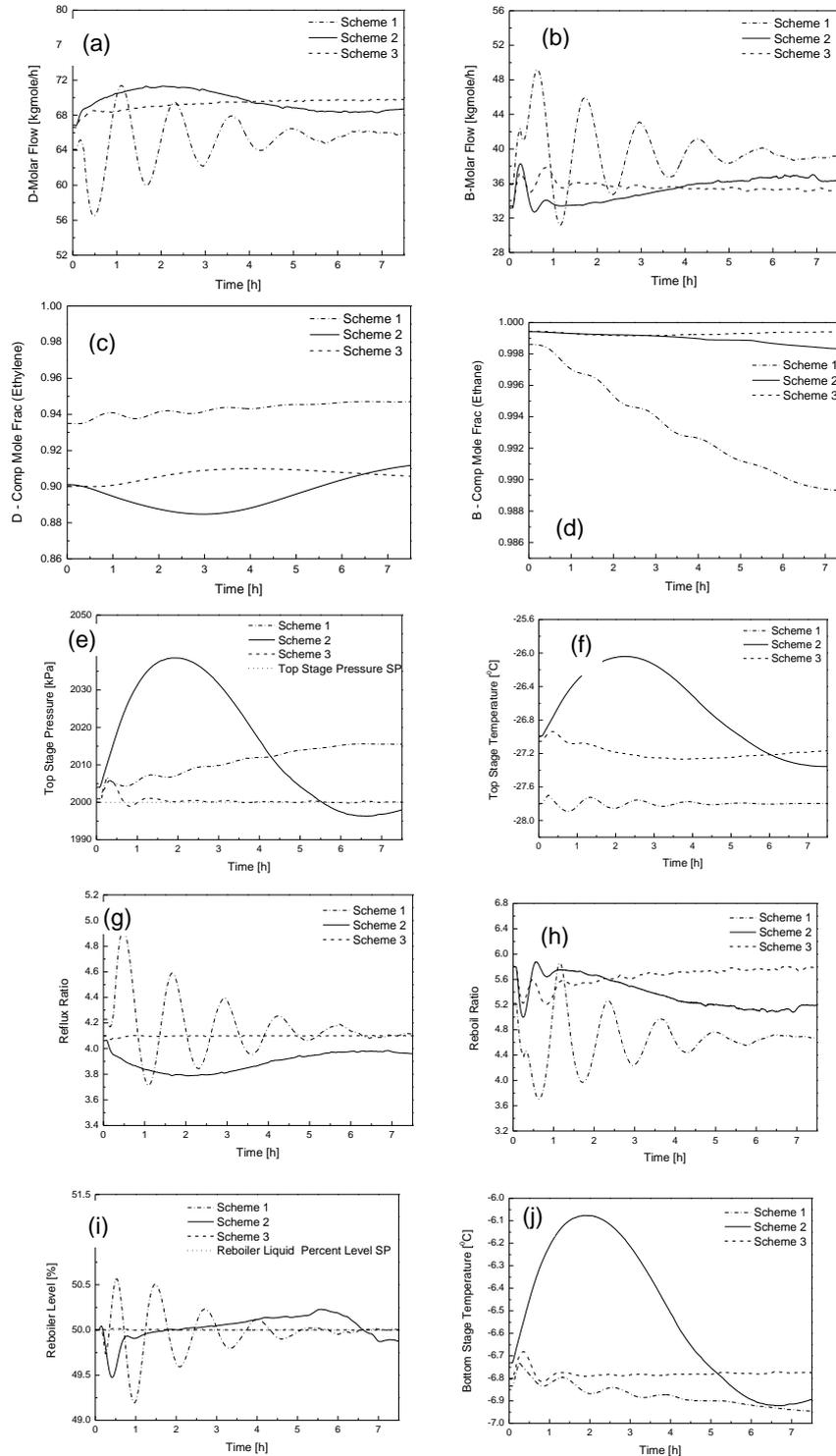
Figure 5: Parameters fluctuation curves of three control schemes for a +5% disturbance in the feed flow rate [(a) distillate flow rate, (b) bottom flow rate, (c) ethylene concentration in distillate, (d) ethane concentration in bottom, (e) top stage pressure, (f) top stage temperature, (g) reflux ratio, (h) reboiler ratio, (i) reboiler level, (j) bottom stage temperature]
