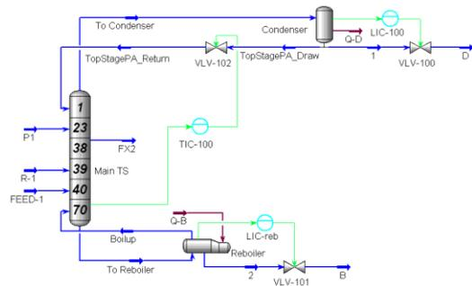
Figure 2: Sub-process configuration of temperature control (S1)
