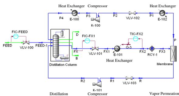
Figure 1: The main control scheme of hybrid distillation-vapor permeation process of ethylene/ethane
