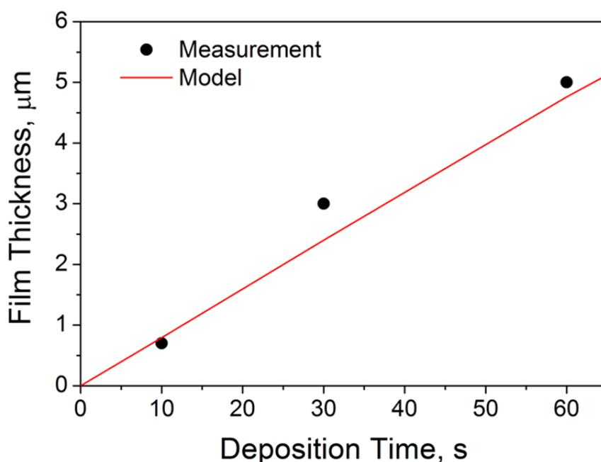
Figure 1: Calculated film thickness (line) and measured film thickness (points) as a function of total deposition time.
