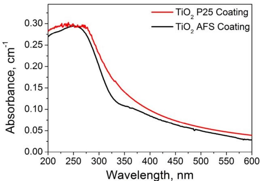
Figure 3: UV-Visible absorption spectra of P25 coating prepared by solvent evaporation technique and AFS  $\text{TiO}_2$  coating obtained with a total deposition time of 30 s.
