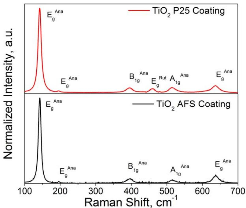
Figure 2: Raman spectra of P25 coating prepared by solvent evaporation technique and AFS  $\text{TiO}_2$  coating obtained with a total deposition time of 30 s.
