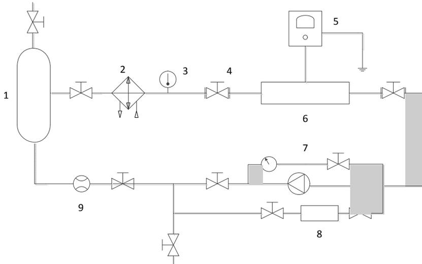
Figure 1: Pipe flow experimental system. 1: stainless-steel vessel; 2: heat exchanger; 3: temperature measuring instrument; 4: insulated flange; 5: pico-ammeters; 6: charge accumulation duct; 7: pump; 8: conductivity measuring cell; 9: flow meters.
