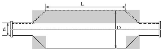
Figure 3: Structure of the electrostatic buffer
