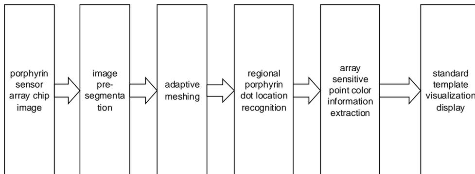
Figure 5: Diagram of image processing
