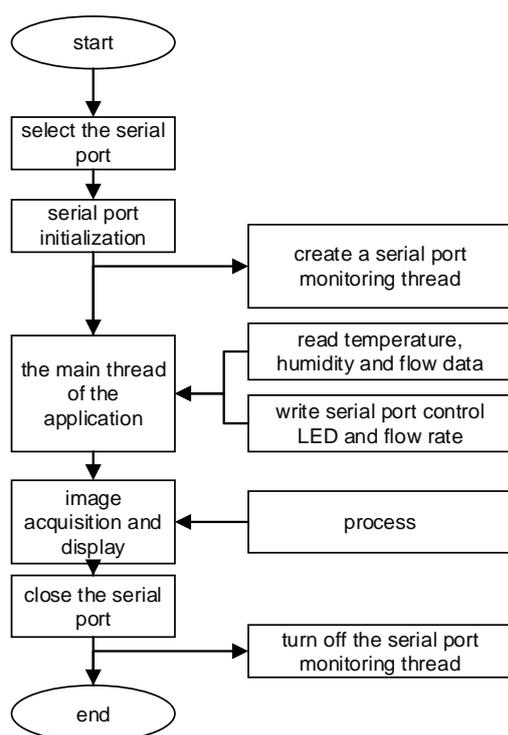
Figure 3: Diagram of serial communication
