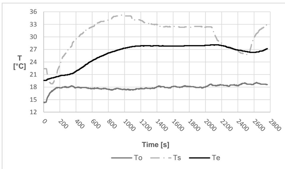
Figure 3: Exhaust air temperature ( $T_e$ ) and supply air temperature ( $T_s$ ) as a function of outdoor air temperature ( $T_o$ )
